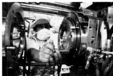
The CDs are injection-molded, one at a time.
