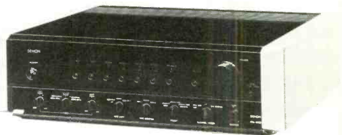
The Denon PRA-6000 preamplifier provides pure non-feedback circuitry from its moving coil head amps through the amplifier section.
