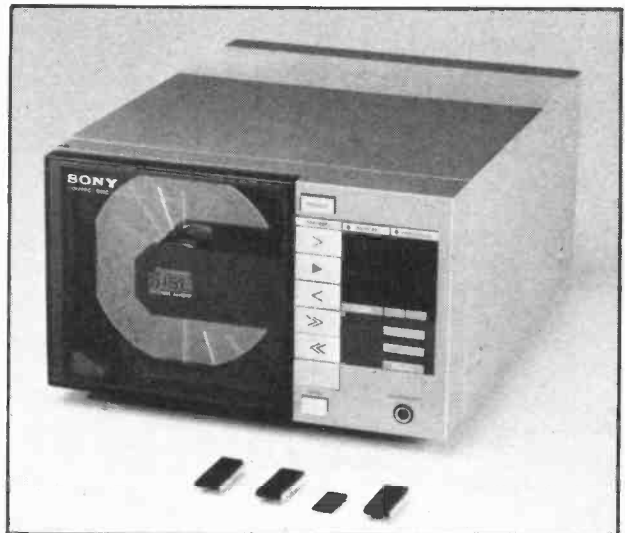
Sony's compact disk player (prototype) with three types of LSI circuits for DAD (digital audio disk).
