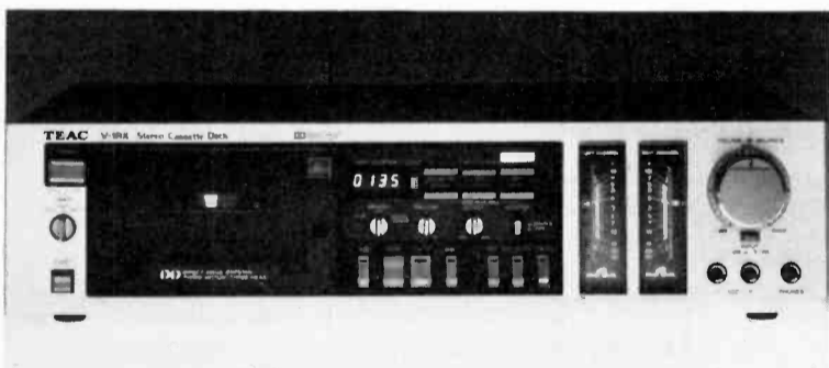
DOUBLY QUIET —The TEAC V-IRX three-head cassette deck offers separate dbx noise reduction systems for record and playback. Claimed wow and flutter on the $590 deck is 0.025%. A "Bias Fine" adjustment control allows compensation between the different bias requirements of various tape brands.
