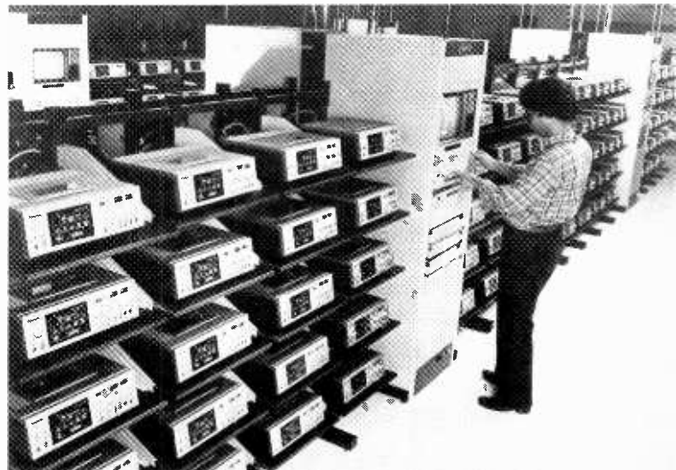
VIDEO VIDEO —A technician adjusts controls in one section of the new Vidtronics Videocassette Division in Los Angeles. On an annual basis at full operating capacity, the facility can duplicate some seven million videocassettes.
