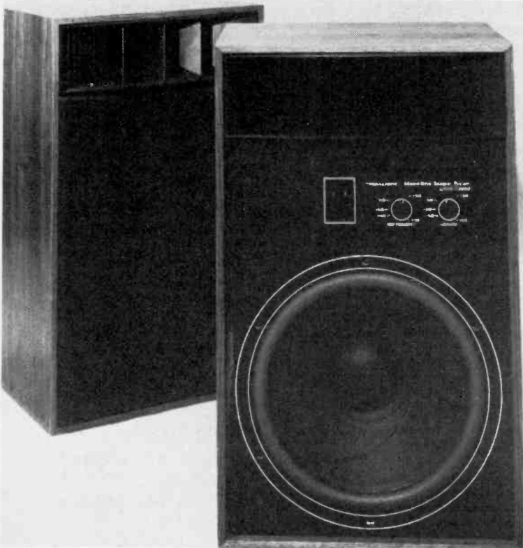
MACH ONE —Radio Shack has developed an improved version of its Mach One speaker system. The unit, called the Mach One Liquid Cooled Speaker, offers a power handling capacity of up to 160 watts with a response of 25-20,000 Hz. The unit is said to use a magnetic liquid that increases its power handling capacity by improving the transfer of heat away from moving driver elements. The liquid, designated "ferrofluid," also helps to control voice coil travel thereby reducing wasted motion. The new Mach One, with a price tag of $239.95, uses a 15-inch woofer, a liquid-cooled sectoral midrange horn and a heavy-duty, liquid-cooled bullet tweeter.
