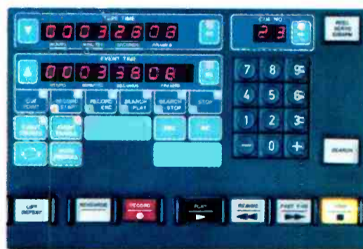
ATR-124's Multi-Point Search-To-Cue (MPSTC). Provides 100 cue locations.
