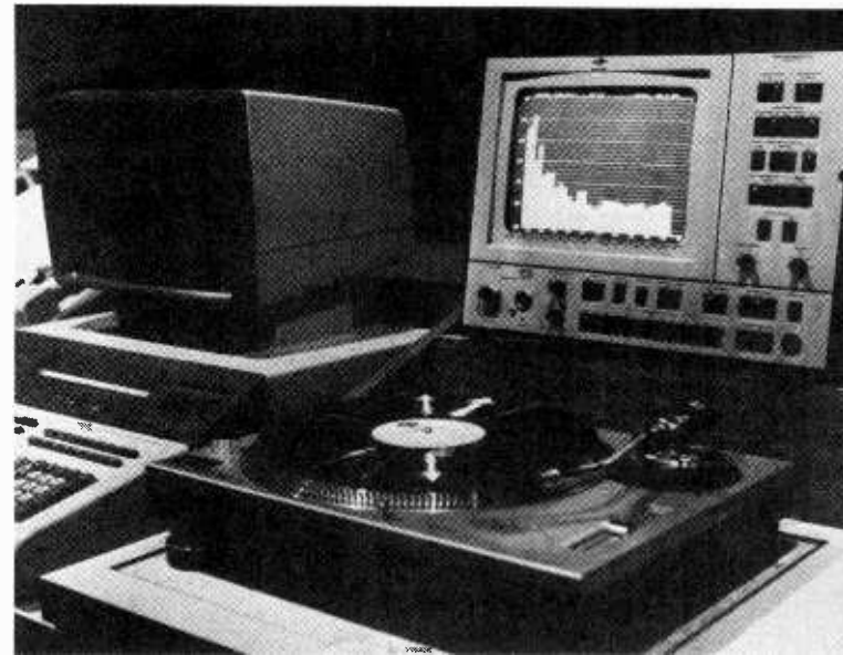
Testing Records: Sophisticated Hewlett-Packard computer at left in a sound evaluation room at Keysor Corp., Saugus, Calif., a leading supplier of vinyl compound to the industry, is able to analyze records with a high degree of sophistication. Firm maintains that this approach and level of sophistication is unique among compound manufacturers.
