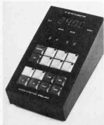
AUDIO KINETICS debuts the XT-24 Intelocator, a microprocessor-based device of control of multi-track tape machines including the 3M M79, Studer A80, Ampex MM1200 and MCI JH-16 units.
