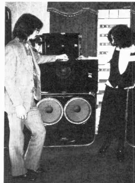
COMMUNITY Light & Sound's Tom Horan, who designed the Zoids line of fiberglass horns, shows off features of the new MB-60 mid-range unit with a 12-inch cone that rounds out the road/disco package.
