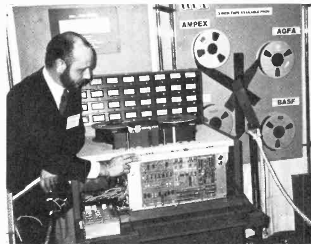
Billboard photos by Stephen Traiman MCI's Lutz Meyer points out electronics and features of the revolutionary 32 track, 3-inch tape, 20 i.p.s. recorder.
