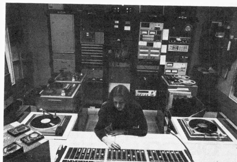
Billboard photo by John Woram WQXR engineer Sandy Singer , flanked by pair of new Panasonic SP-10 Mk-2 turntables, demonstrates new McCurdy console in main control room.
