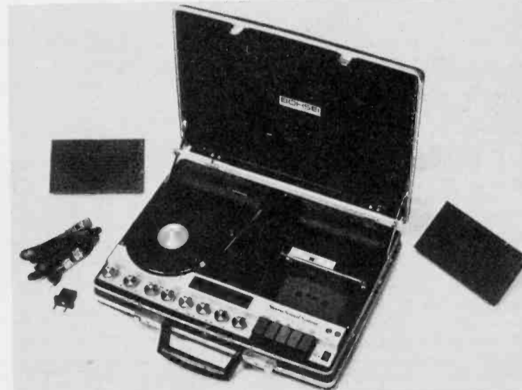
COMPACT STEREO system in slim attache case is one of the initial products introduced by Bohsei Enterprise Co. USA. Model ARC 6100 has AM/FM radio, 3-speed phonograph, and cassette tape recorder/player with remote speakers. Suggested list: $149.95.
