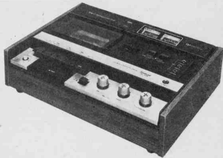
SPECIAL HEAD of magni-crystal ferrite is one of the meticulously crafted elements in the hand assembled Sansui stereo cassette deck model SC 363. Four-pole hysteresis synchronous drive motor and safety devices to prevent tape jamming, breakage, stretching, or accidental erasure are also featured. Photoelectric sensor shuts tape off automatically. Suggested list: $279.
