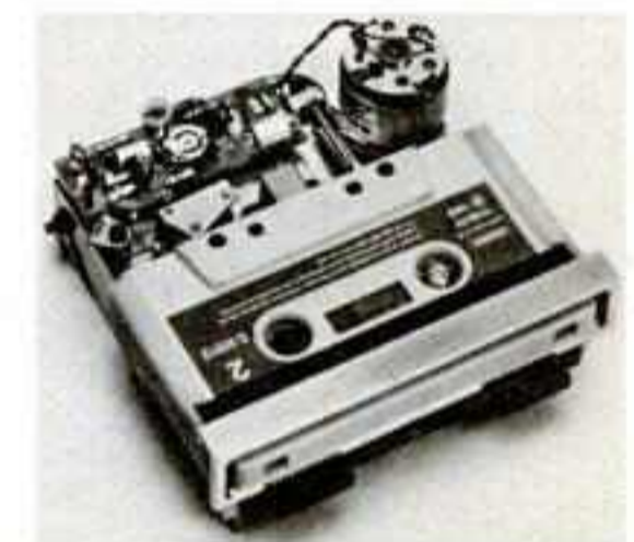
SUPER MINI AUTO CASSETTE PLAYER was introduced by Staar to comply with strict size regulations expected in Europe for 1975. The unit is 1½ ins. high, 4 ins. deep and 4¼ ins. wide.
