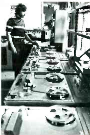
Duplicating for 140-plus stations is no simple chore. Here, Ron Manly guides five high-speed duplicating machines located at the Watermark headquarters.
