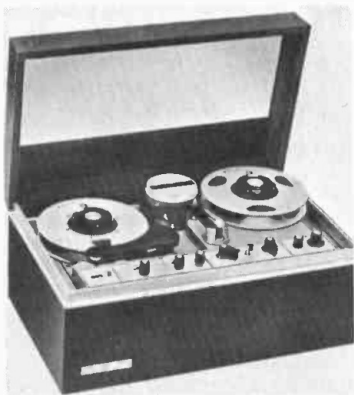
BELL & HOWELL'S new video tape recorder, shown above, is available in both black and white and color versions. The monochrome unit, priced at $1,835, can be converted to color by adding one plug-in circuit board. Both units feature helical scan, have a playing time of one hour with 2,150 feet of one-inch tape and weigh 47 pounds with carrying case.
