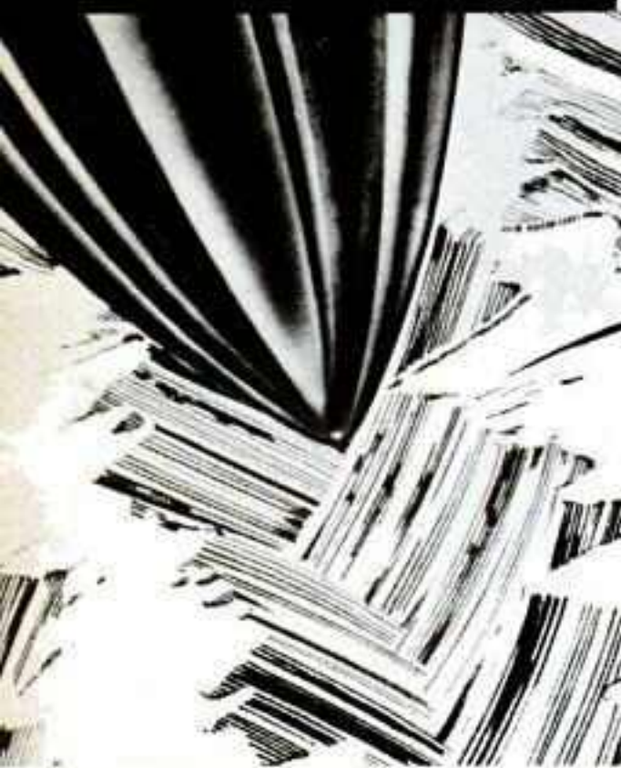
Diamond needle in record groove
