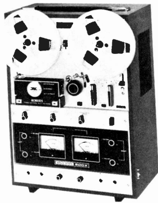
MODEL 800X. This new tape recorder by Roberts, a division of Rheem Manufacturing Co., boasts 40 watts peak power, and has an automatic reverse feature which provides for continuous playback in both directions of 12.8 hours of uninterrupted music. The 800X also features sound-on-sound, which adds sound to prior recorded material, on a separate track, without erasing the previous recording. Its recommended list price is $539.95.
