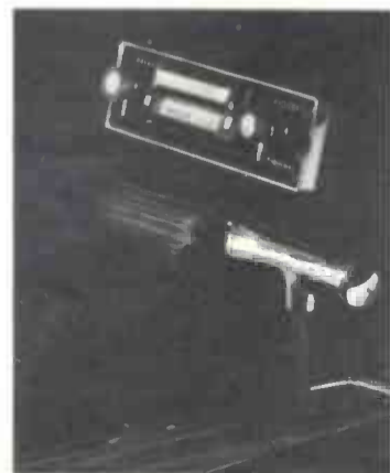
THE NEW Philips stereo car cassette playback unit is self contained, fully transistorized and operates on a 12-volt car battery. Selling price is $129.95.
