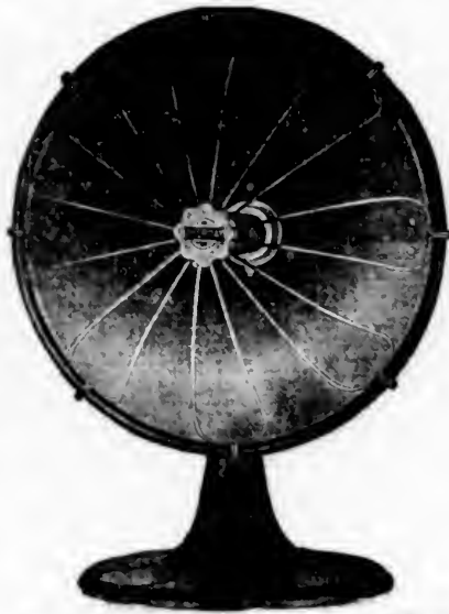
No. E3952—Radiator, Burnished copper reflector back and base bronze enameled finish. Screw base element. Heavy wire removable guard. Height, 18 in. Diameter of reflector 12 inches. Complete with 6-ft. connecting cord and separable attachment plug. Watts 600. Weight packed 8 pounds. Each ..... $6.00
