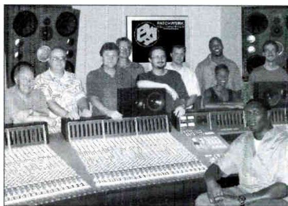
Atlanta Falcons offensive tackle and PatchWerk Recording Studios owner Bob Whitfield (seated) at the recently installed, 80-channel Solid State Logic 9000 J Series console.
