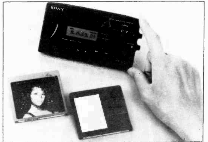
Prototype of Sony's Mini Disc player/recorder; (bottom, l-r) prerecorded Mini Disc and blank recordable Mini Disc.
