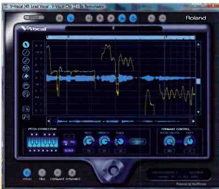
Cakewalk's SONAR comes with the Roland V-Vocal plug-in, which offers pitch correction and shifting, formant control, and more.
