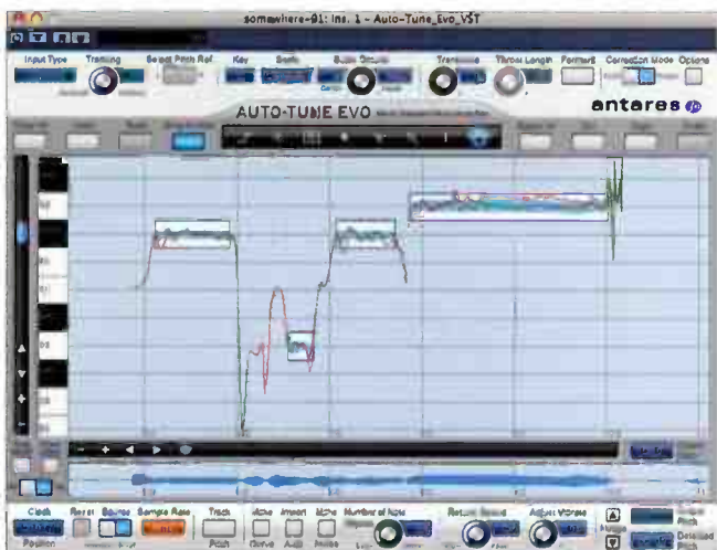
Auto-Tune's graphic mode lets users "draw" in pitch correction on a note-by-note basis.
