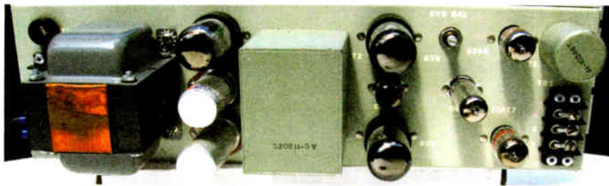
A control to adjust cathode voltage of the 6V6 output stage was the only tweak to tune up the Sta Level.
