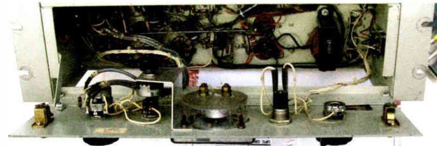
By changing the values of two resistors, the recovery time of the Sta Level could be increased or decreased.
