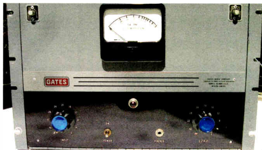
Introduced in 1957, the SA-39B was marketed as a peak level solution for AM, FM and TV stations.
