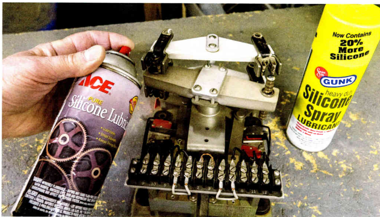
Fig. 1: Silicone spray can be used on RF contacts.
