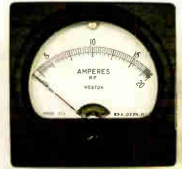
Fig. 4: Thermocouple ammeters are often used to measure RF current.
