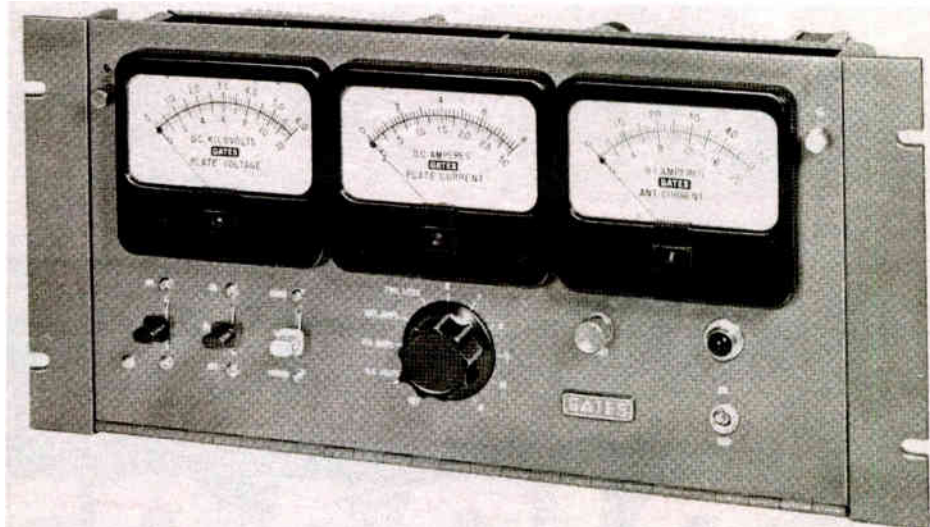
The Gates RDC-10AC is typical of first-generation remote controls, with 10 metering/control channels accessed by stepping relays in the studio and transmitter units. Two phone lines with DC continuity were required for control and metering.
