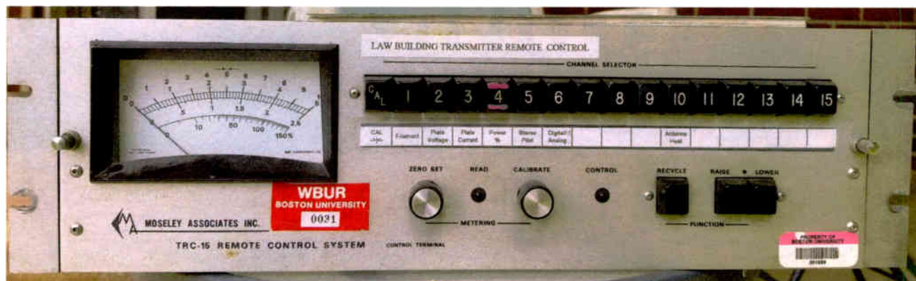
Introduced in 1975, the Moseley TRC-15 used digital techniques to eliminate stepping relays.
