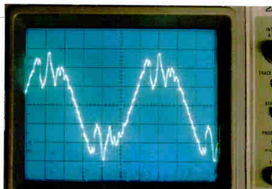
Fig. 6: A Winco PSS8000 generator ragged waveform.
