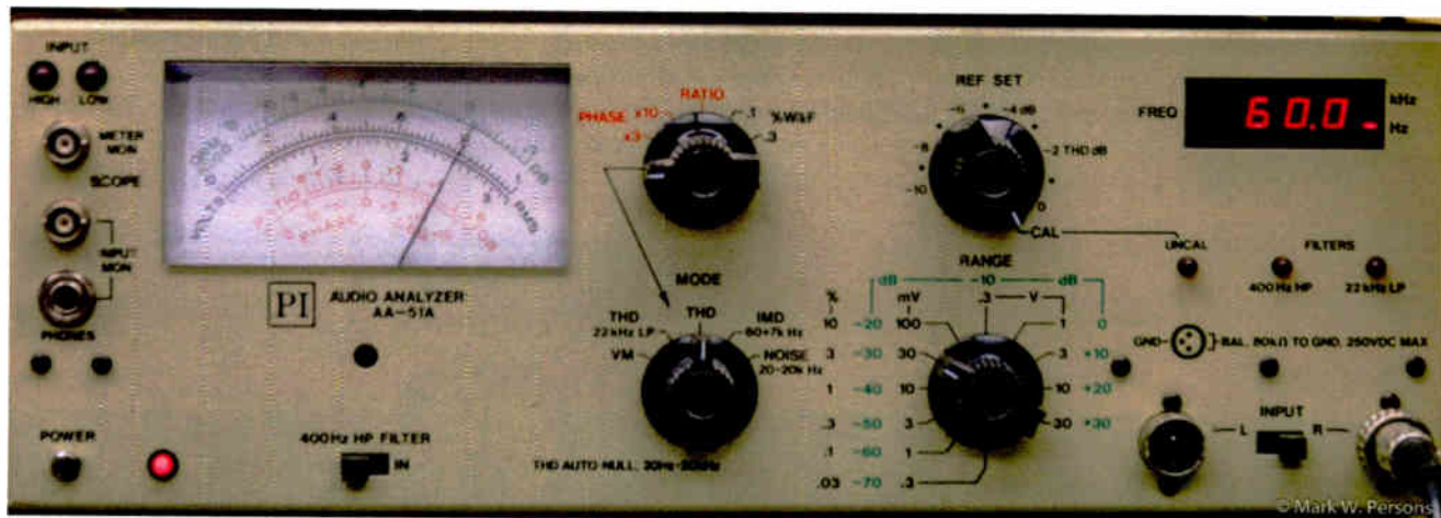
Fig. 4: Harmonic distortion 2.5 percent on generator at 60 Hz.
