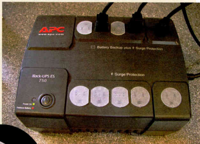
Fig. 3: Child-proof safety caps dissuade unauthorized AC use.
