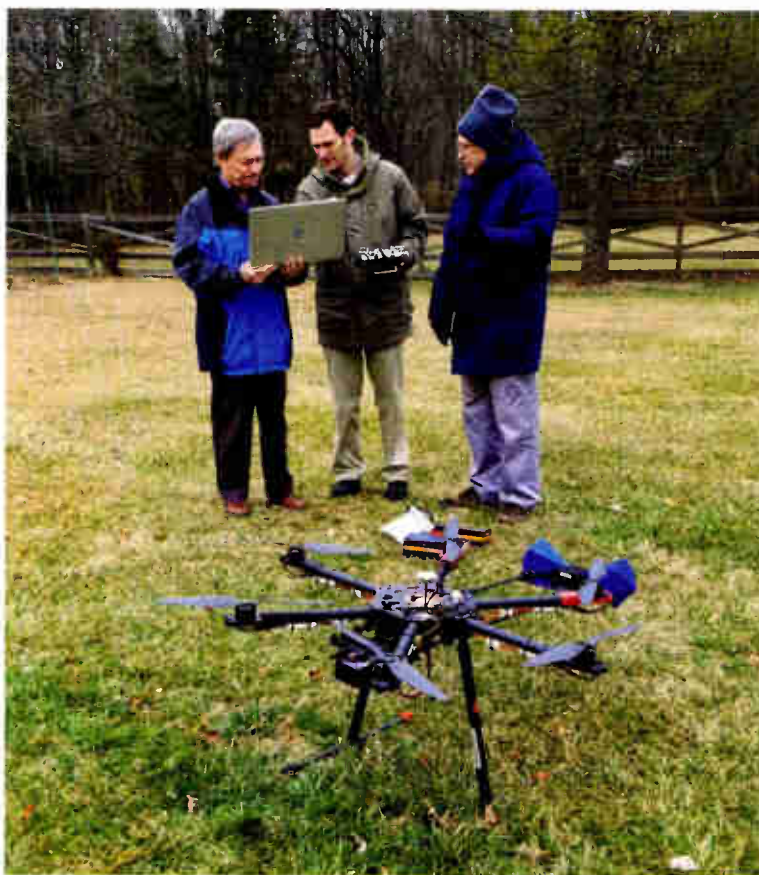
Among regular projects at Cavell Mertz, Kean has helped in the development of an RF measurement drone, which provides precision measurement of television and FM signals from transmitting antennas. This was presented at the Broadcast Engineering and IT Conference. Here the vehicle is shown in early flight testing.
