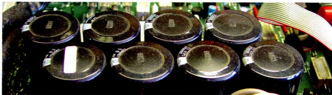
Fig. 1: Note the "domed" tops of these "bad" capacitors.
