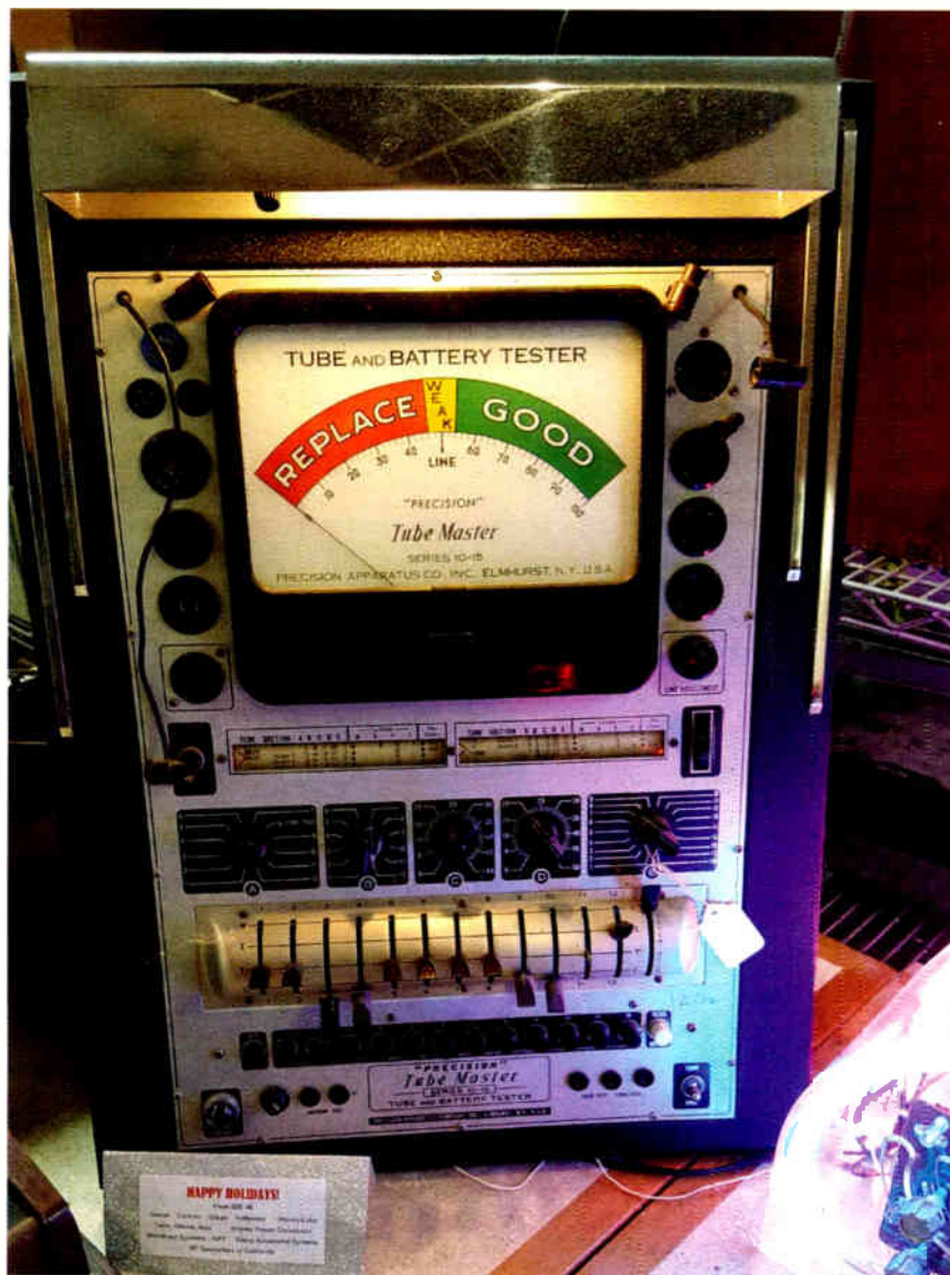
Fig. 4: When most electronics operated with tubes, a tube checker like this one was commonplace.
