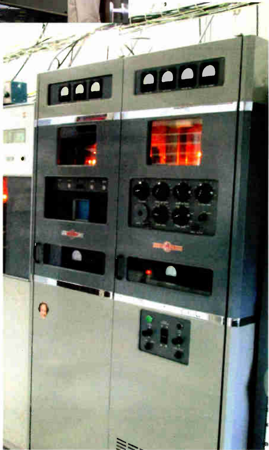
Moersdorf's collection contains only one non-broadcast transmitter, this Collins AN/FRT-24 1 kW base station transmitter built for the U.S. Navy. It tunes 2-30 MHz and was constructed in the mid-1960s.
