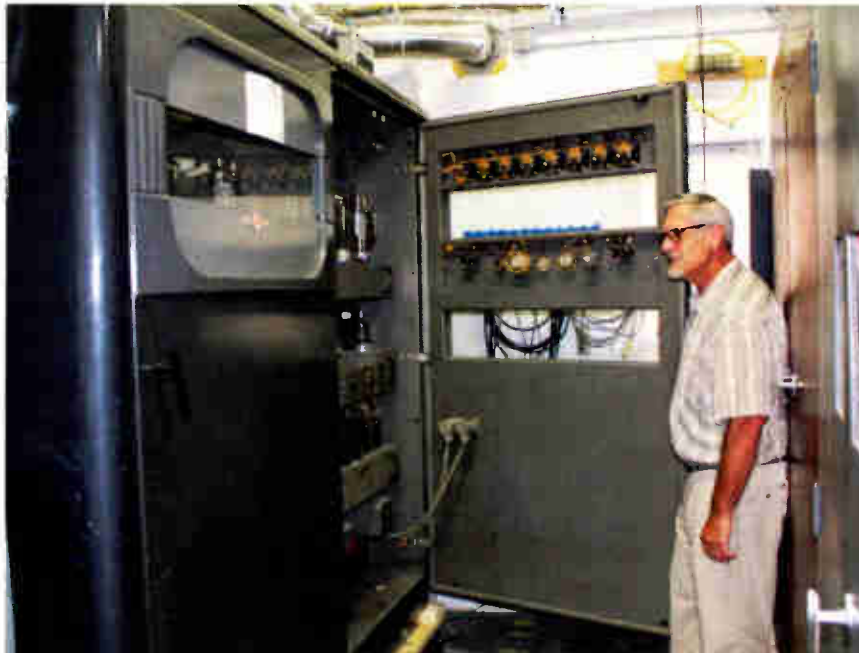
Moersdorf and his "Big Bertha" 1946 Collins 20T. It was designed for 1 kW operation and weighs in at a whopping 5,700 pounds. (That's less than 0.2 of a watt per pound.)
