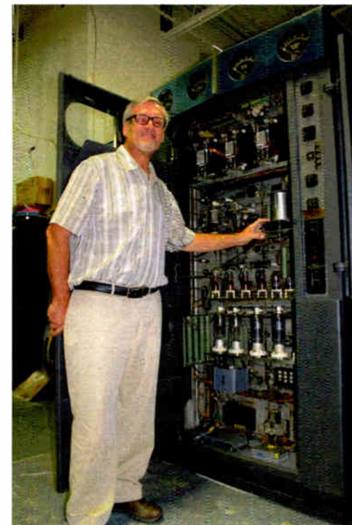
Gerry Moersdorf shows off the oldest item in his large collection of broadcast transmitters. The Western Electric 443A1 1 kW Doherty dates to the 1940s. Moersdorf notes that it tunes between 550 kHz and 2,750 kHz, allowing it to be used in the old police band for one-way "broadcast" communications.
