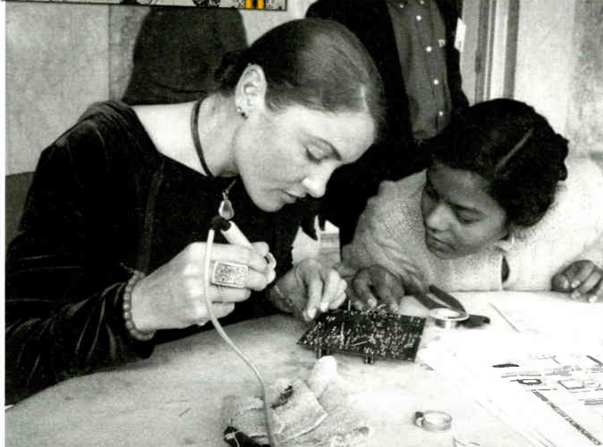
Women solder a transmitter board in Nepal in a photo from "Low Power to the People." Volunteer photo/Prometheus Radio Project, reprinted courtesy of The MIT Press.
