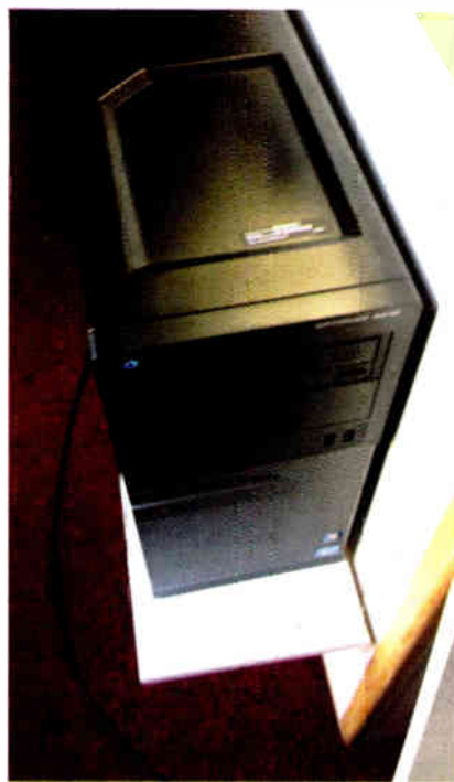
Fig. 2: If the computer tower is enclosed, the shelf helps avoid cooling problems.
