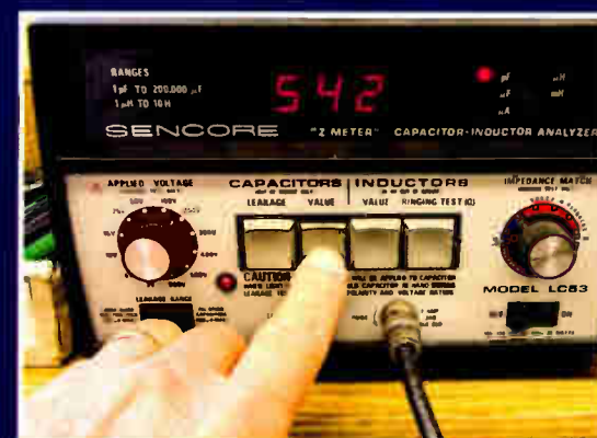
Fig. 7: Measure capacitance to confirm it is right.
