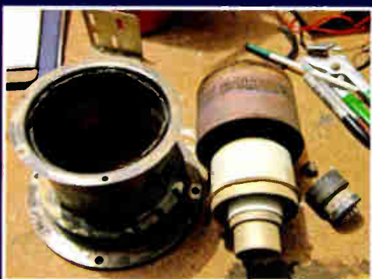
Fig. 2: These items have overheated.
