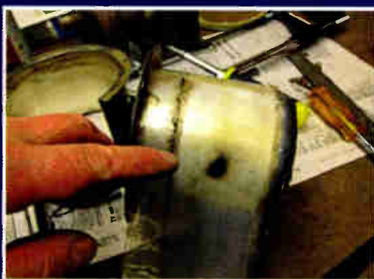
Fig. 4: Note the arc-over spot.
