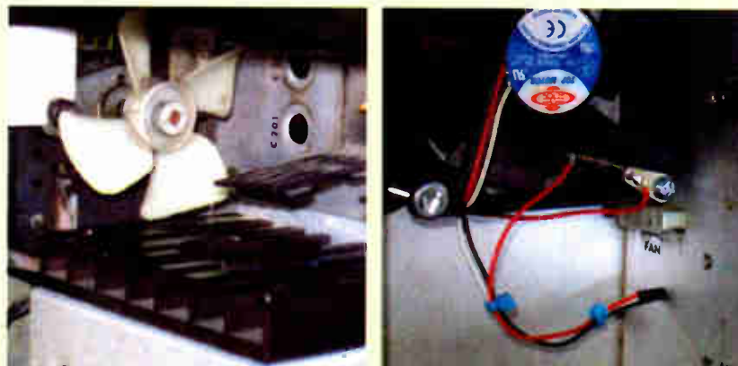
Fig. 1: The Marti STL-8 with its AC cooling fan.
