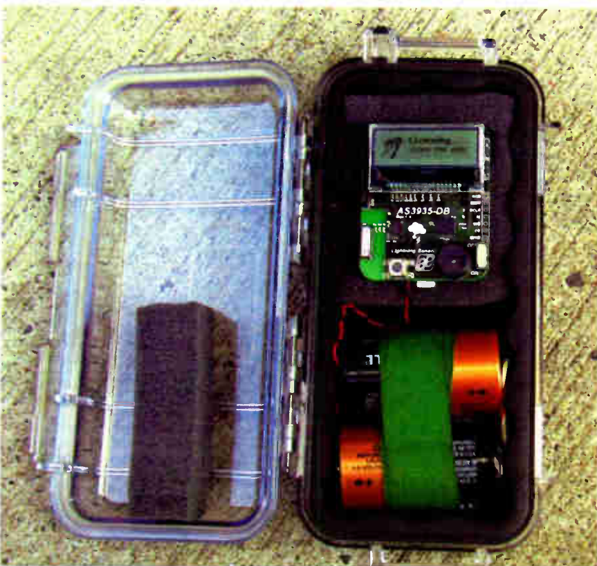
Fig. 5: The detector was modified to operate with "D" cells.
