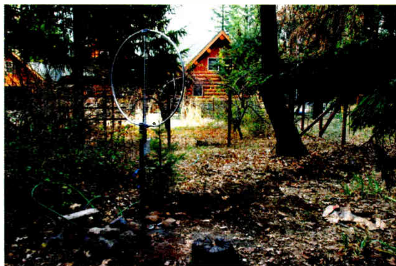
Dave Hershberger told the FCC: "The main problem with AM radio is that it only works in cars anymore." He installed a Pixel Technologies broadband loop antenna to pull in the signal from KNCO(AM), Grass Valley, Calif., six miles from his home.
