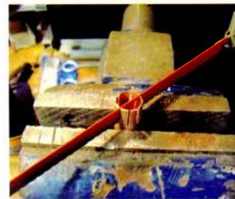
Fig. 7: Serrate an edge of the copper support pipe.
