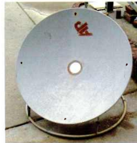
Fig. 6: Fasten the filler panel to the dish, using four #6x32 bolts and nuts.
