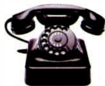
1936: The advent of the dial desk phone. No more asking the operator to connect you.
