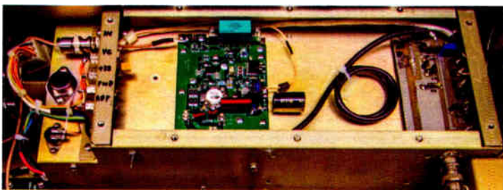
Fig. 2: The new pallet amplifier, inside the 802A.
