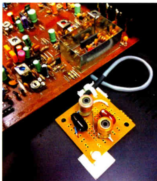
Fig. 3: Paul built the circuit on a perfboard and mounted it inside the receiver.
