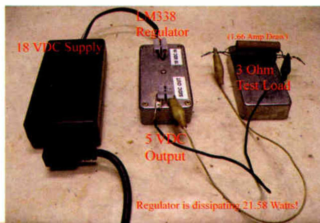
Test Setup using series Rectifiers in front of LM338 Regulator
