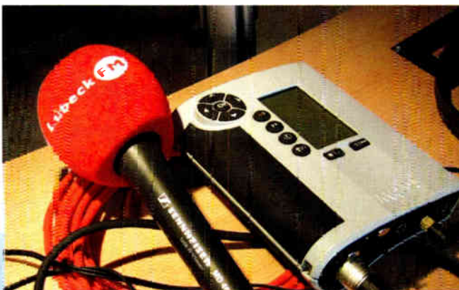
The Lübeck FM portable rig: a microphone and Mayah Flashman II codec/recorder.
