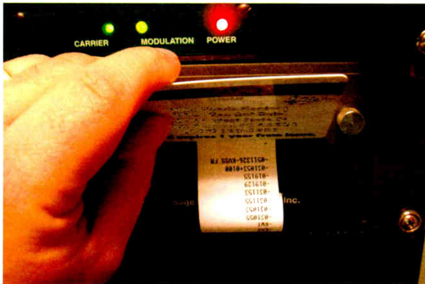
Fig. 1: An old plastic phone card saves the Sage printer mechanism.
