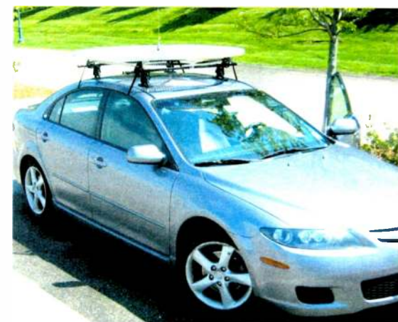
Fig. 3: Calibrated vertical ground plane antenna on the vehicle used for Rhode Island testing
