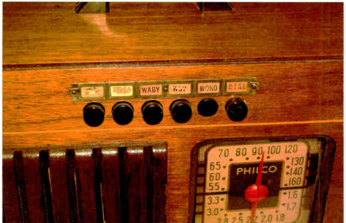
Fallout from the frequency shift affected another U.S. sector: the radio serviceman. An estimated 10 million sets with push buttons needed resetting, offering an unprecedented opportunity to cash in. (The majority of radio owners were not about to tweak oscillator and RF stage trimmers to bring in the new frequencies.)
