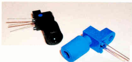
Left: Fig. 1: A simple fiber optic encoder/decoder gets an alarm across an AM tower base insulator.
