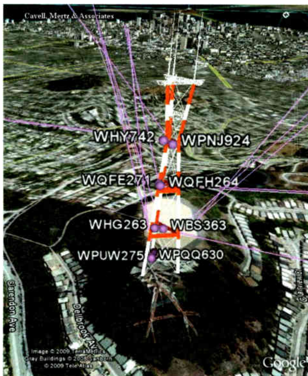
Fig. 3: The marriage of data with Google Earth offers a unique interpretation of the 7 GHz links at San Francisco's Sutro tower, courtesy of Cavell, Mertz & Associates.
