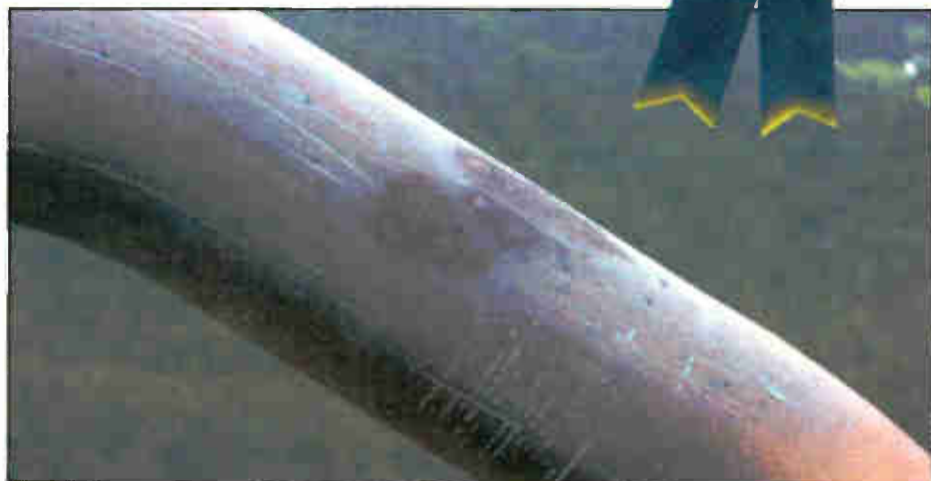
Fig. 1: Lightning hit this top FM bay, pitting the surface and causing an arc within — note the discoloration due to heat.
