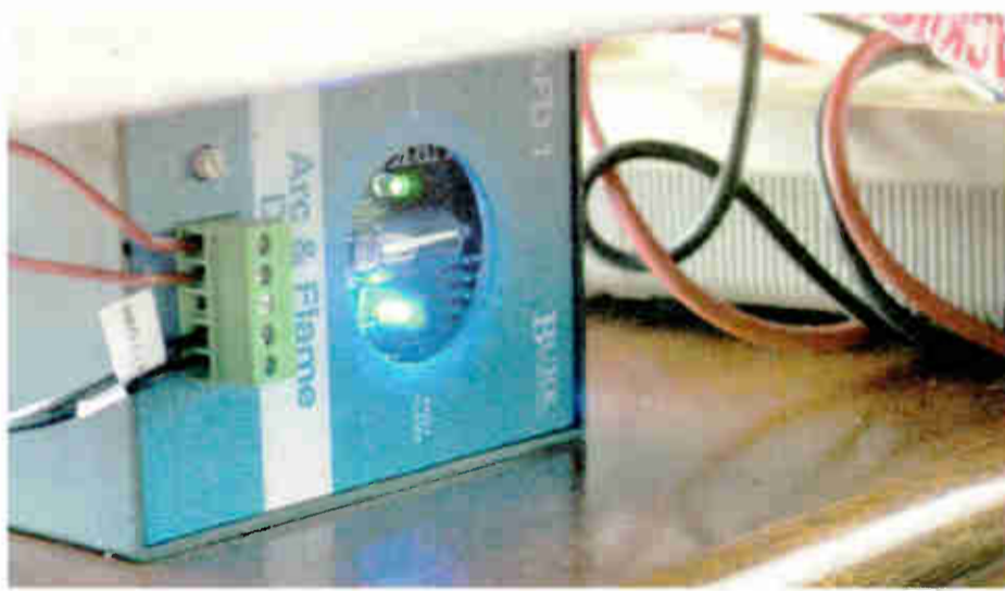
Fig. 2: The AFD-1 senses the flame from across the room to trigger an alarm.
