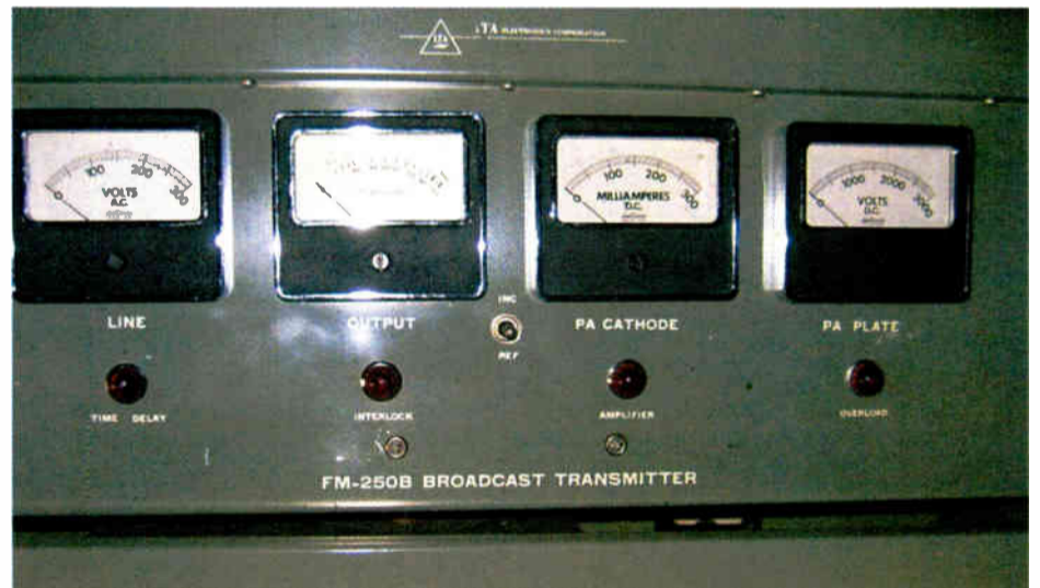
After replacing broken meter glass and a thorough cleaning, it is starting to look respectable.
