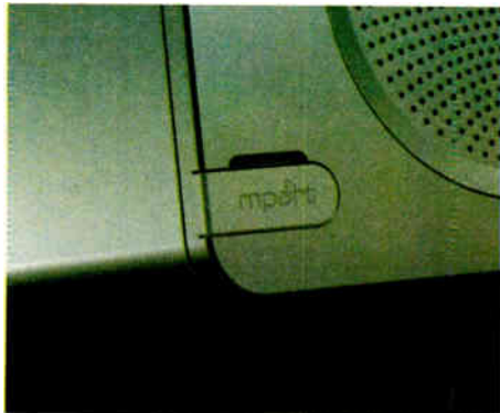
The M-Port female miniature jack, under this rubber tab, accepts an input from an MP3 player.
