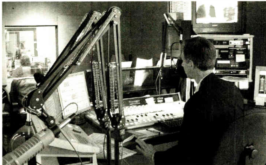
Morning host Ken Lass at the Wheatstone G6 Control Surface in WDJC's control room. The studios are in a line, with windows between, so that you can see through the receptionist's area and into the WXJC control room,' said Poole.
