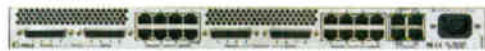
88 I/O CONNECTIONS: E 2 has both DB-25s for punchblock interface and RJ-45s for point-to-point interface. All SQUARES have 12 individually configurable opto-isolated logic ports that can be either inputs or outputs.
