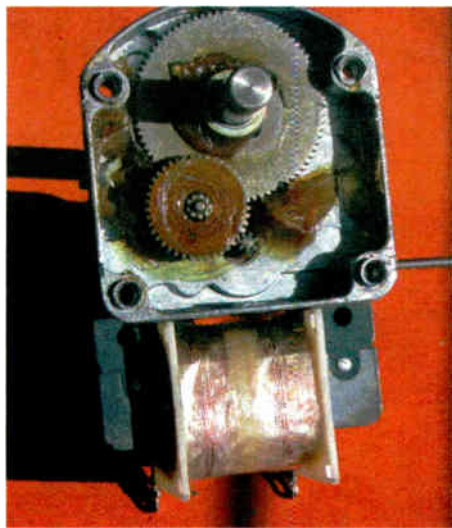
Fig. 3: Dried grease can cause sluggish operation.
