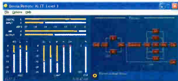
The processing paths of an AM station are shown on this screen shot of an Omnia5.EX.
