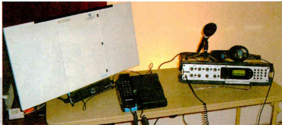
Most of the same gear, organized more neatly and photographed at the author's house. From left: the Thrane & Thrane folding satellite dish; Thrane & Thrane satellite phone; Telos Systems Zephyr Xstream MXP ISDN; and (on top of the ISDN) an Electro-Voice RE50 microphone and Sony 7506 headphones.
