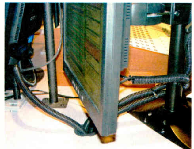
Fig. 4: Black plastic jackets help organize a multitude of monitor cables.
