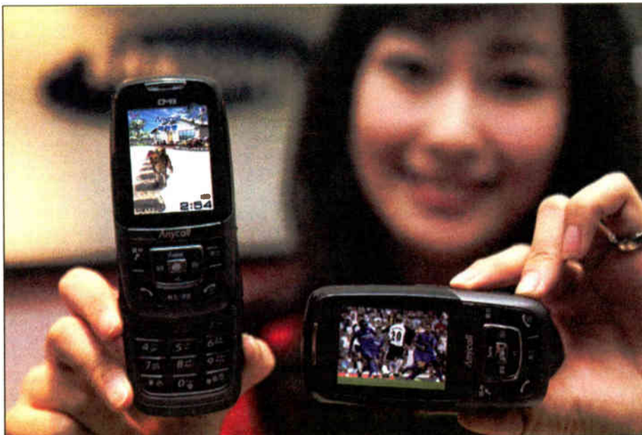
DMB uses Eureka-147 DAB-based technology to deliver video, images, audio and text to portable receivers, including mobile phones such as this Samsung SCH-B360.
