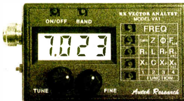
Fig. 3: The Autek VA1 helps determine impedances.
