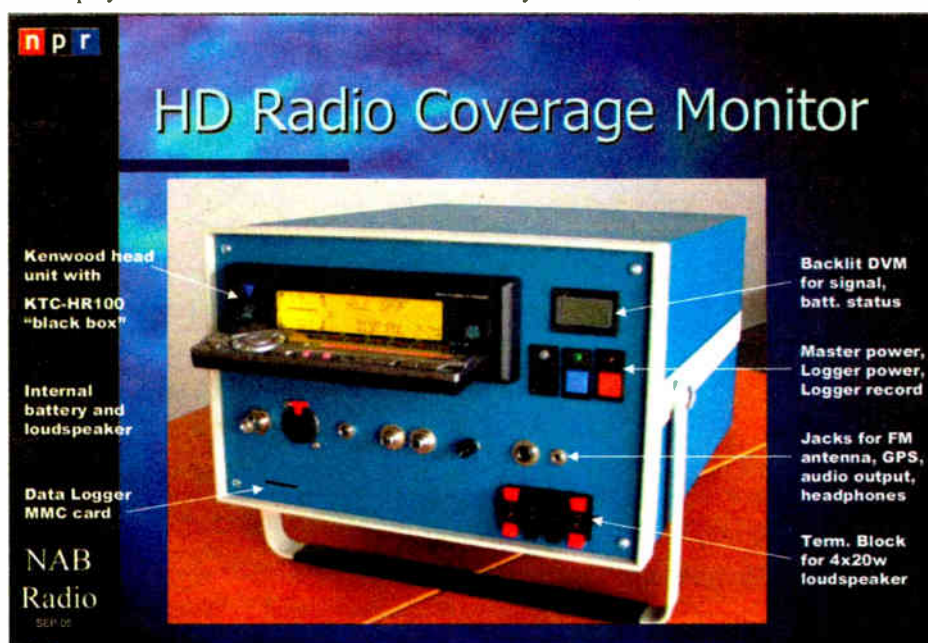
NPR is using this monitor to map HD-R coverage.
