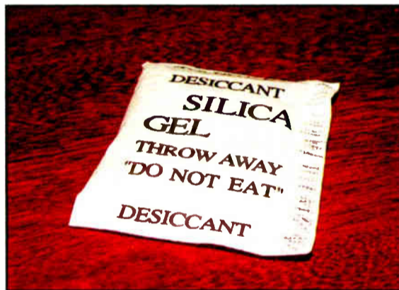
Fig. 4: Use silica gel packs to ward off moisture damage.
