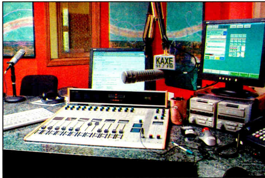
KAXE's Mosaic control surfaces are configured with 12 Penny & Giles faders in modular blocks of two.
