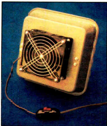
Rear view showing the muffin fan mounted on the cake pan.
