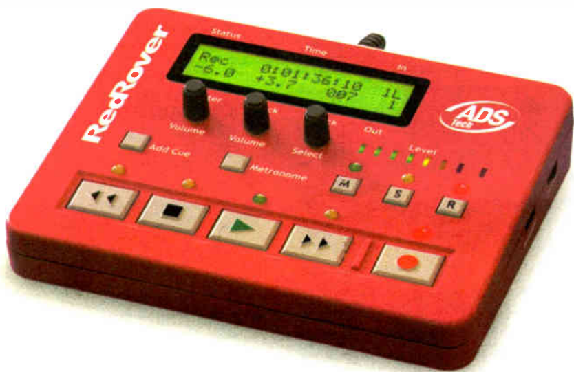
Fig. 1: The Red Rover interfaces to Cool Edit Pro 2.0 and higher to provide remote control of the device.
