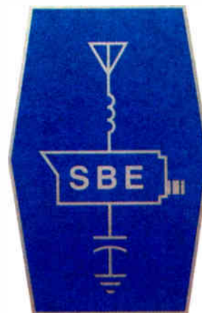
Four schematic symbols, from top, appeared in the original logo: antenna, inductor, capacitor and ground potential. The drawing around the letters is an outline of a TV camera.
