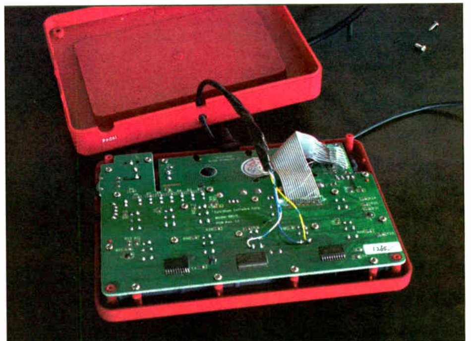
Fig. 2: Solder parallel wires across the control switches to permit console interfacing to the Red Rover.
